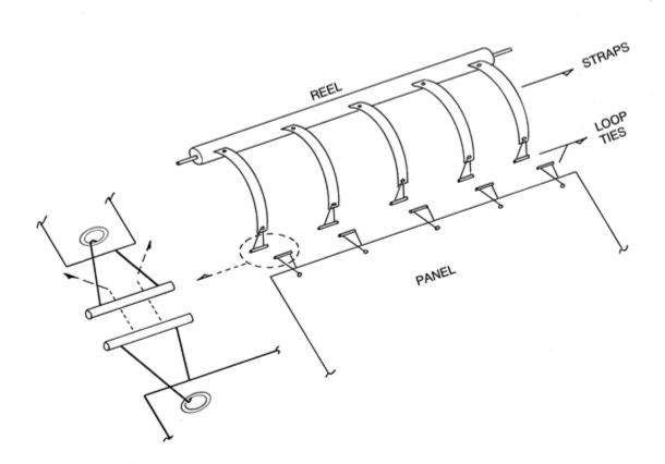
The diagram above shows the typical attachment of a blanket to a winder reel. The loop ties attached through the grommets in the blanket are "twisted" through the loop ties in the lead straps, which are mounted to the winder tube.
