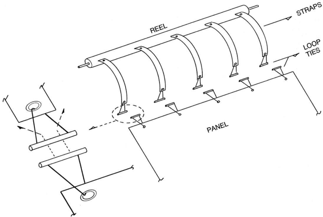
The diagram above shows the typical attachment of a blanket to a winder reel. The loop ties attached through the grommets in the blanket are “twisted” through the loop ties in the lead straps, which are mounted to the winder tube.
