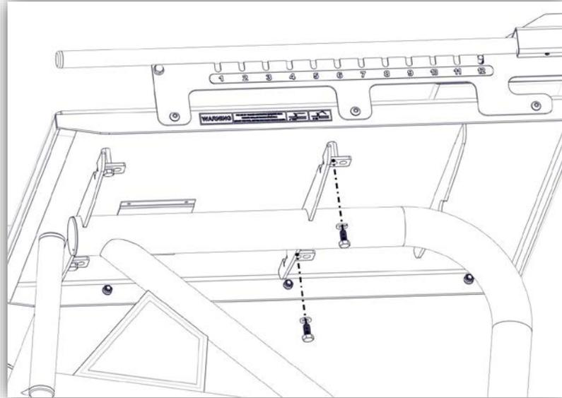
2. Place attachment loops on underside of weldment on the starting platform frame as shown. This step may vary based on the starting platform used for installation.
