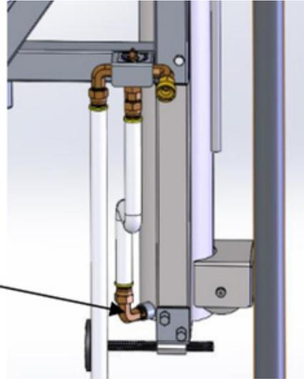
4. Remove Small hose and fitting from cylinder. Replace with new fitting and hose.
