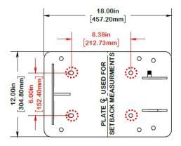
Retrofit Hole Pattern Installations: Use either of the two hole patterns shown below if replacing an existing swim lift on a pool deck. Utilize the hole pattern that matches your existing anchors. ½"-13 mounting screws provided are intended for new anchor installations. Mounting hardware length may require variance for existing anchors.
