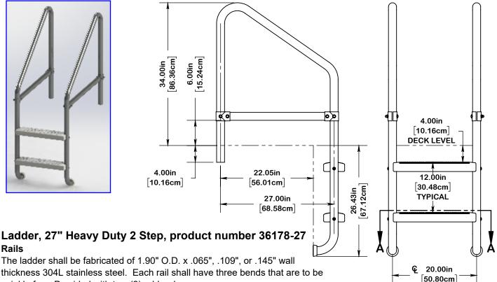
Rails The ladder shall be fabricated of 1.90" O.D. x .065", .109", or .145" wall
