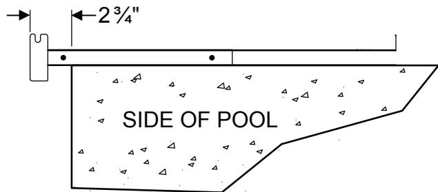
Look through the holes in the base and align the base(s) with your anchor marks.
